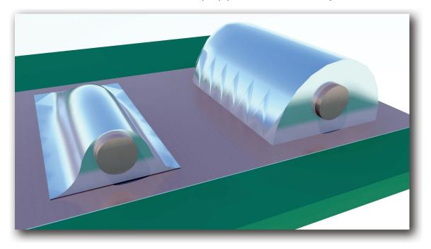
This next illustration shows the range of solder joints one could expect in inspecting a circuit board.
