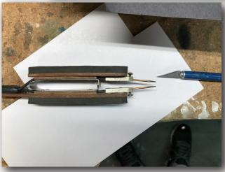
You can't get shocked because the voltage is too low to do much damage, but the tips do get very hot very fast. Not show above is the real magic part: the foot switch. You clamp the parts together with the tweezers, when it looks right, you step on the foot switch to heat the
