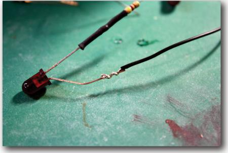
LED leads are pre-tinned and are sharp-edged which grips the wire that's twisted around the lead before soldering. For this application, Iron goes on the bottom and solder goes on the top. I use a temperature controlled Weller conventional soldering station.
